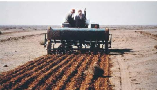
*In the degraded grazeland, machinery introduced by the Project for direct sowing improves rain water infiltration in the soil*
