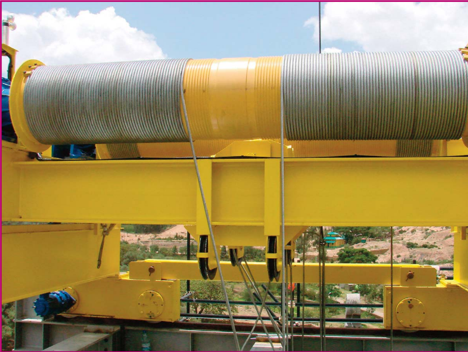
FIGURE 46 – THE BRIDGE CRANE WINCH.
