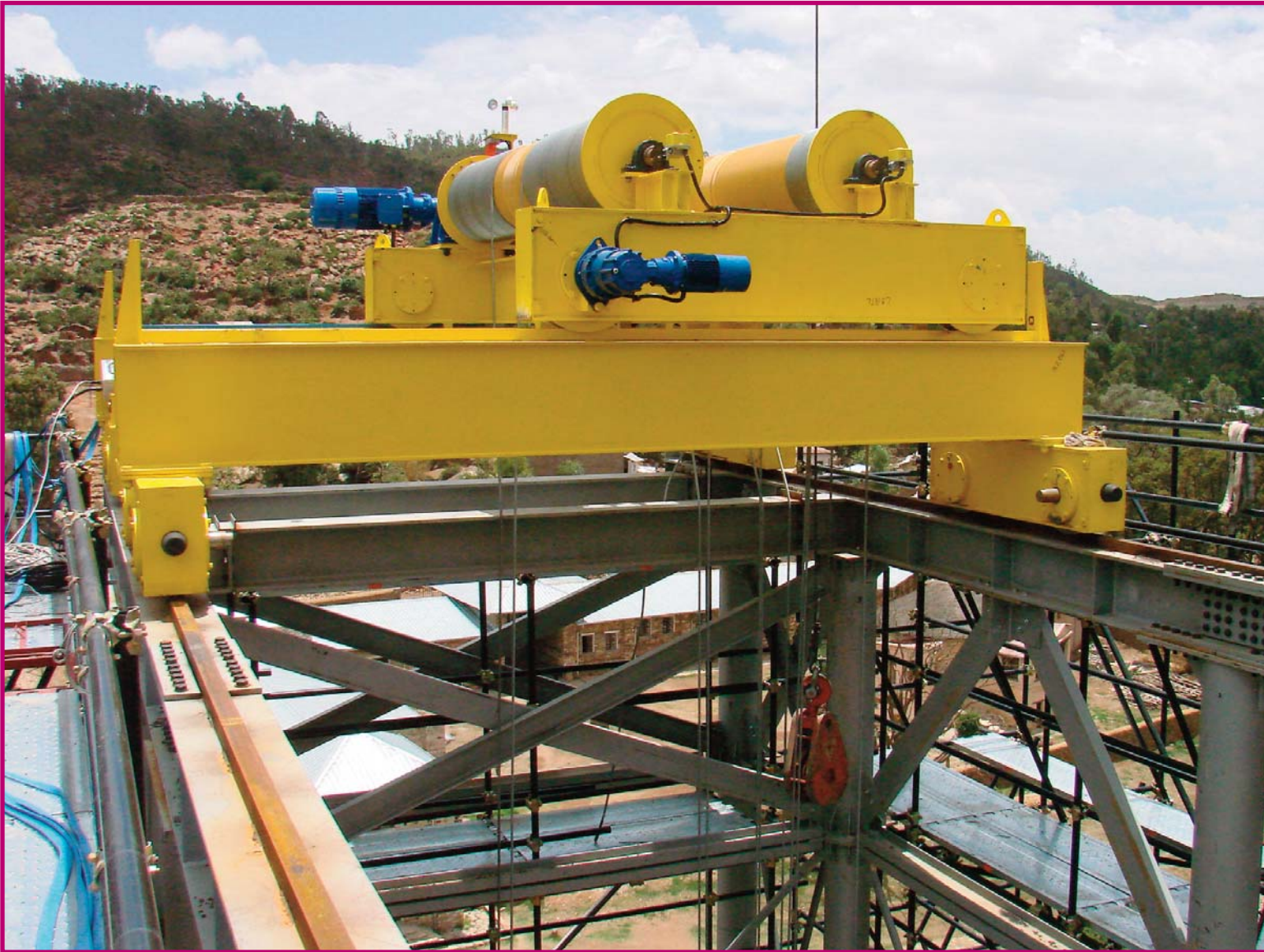
FIGURE 45 - THE BRIDGE CRANE.
