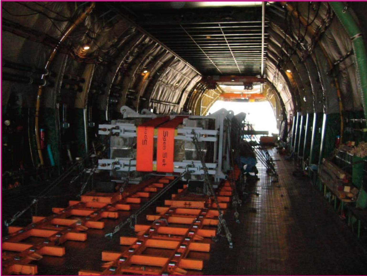
FIGURE 26 – THE ANCHORAGE OF THE BLOCK TO THE AIRCRAFT INTERIOR STRUCTURE
