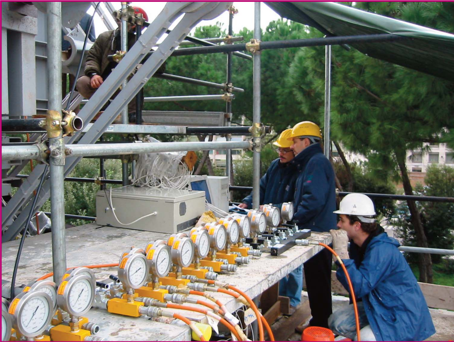
FIGURE 18 – THE MANOMETERS CONNECTED WITH THE JACKS TO CONTROL ALL THE FORCES IMPOSED TO THE STRUCTURE
