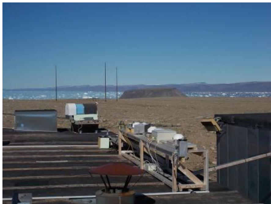
Radiometers and microwave radiometer for the investigation of the atmospheric composition and radiation on the roof of the Thule High Arctic Atmospheric Observatory.
