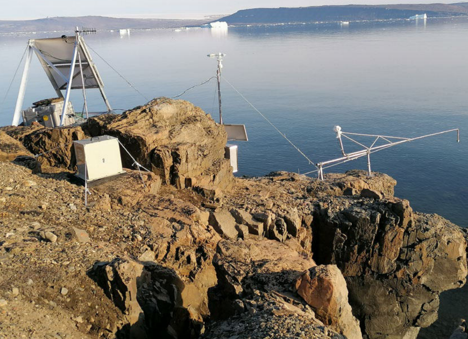
Seismic and tide-gauge station along the Wolstenholme Fjord, north of Pituffik, Greenland (credits INGV and ENEA)
